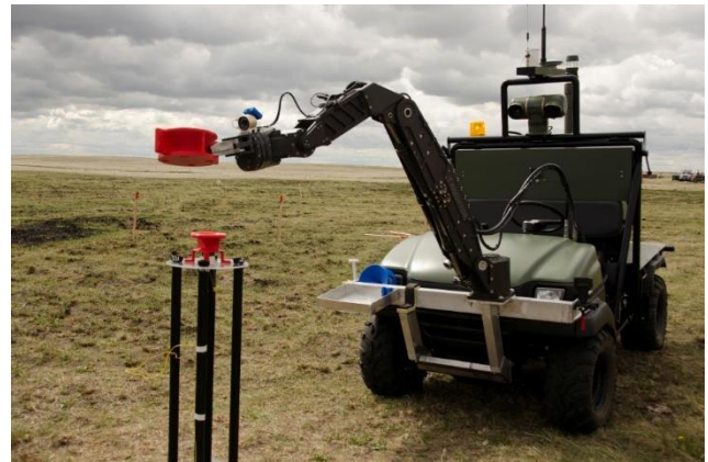
3 – PHOTO: This MATS vehicle, equipped with a robotic arm, handles a highly radioactive material used for a trial at DRDC – Suffield Research Centre . The MATS system allows the operator to stay a safe distance away during manipulation of the source.
