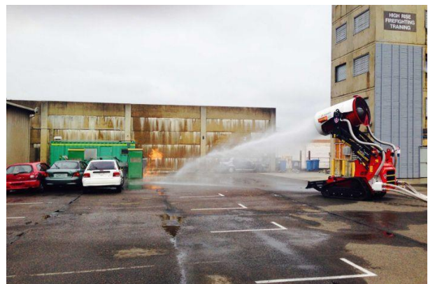
1 - PHOTO: The TAF 20 firefighting robot can blast water up to 90 metres and spray water mist or foam for 60 metres. ( ABC News: Brigid Glanville )
