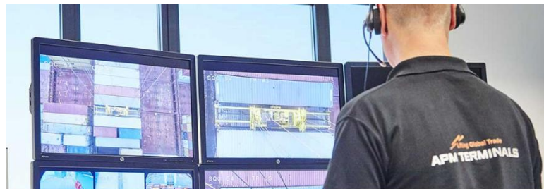
4 - PHOTO: Remote crane operation is an integral part of automation, an important component for marine terminal operation. This improves safety, working environment and overall operator productivity in container terminals. ( ABB )
