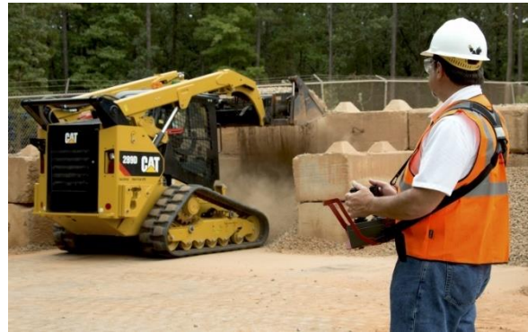
2 - PHOTO: Caterpillar's 'RemoteTask' system allows operators to remotely control construction machines with precision using a 'belly box' control system.
