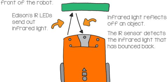
Using EdBlocks, we can write a program that tells the IR LEDs to send out infrared light. If any of that light is reflected off any objects nearby, it will bounce back towards Edison. Edison can detect that light with the IR sensor.
